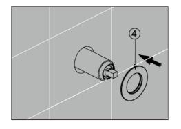
2. FIXING THE VALVE BODY
